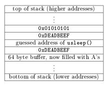
Figure 2: Stack after one probe
